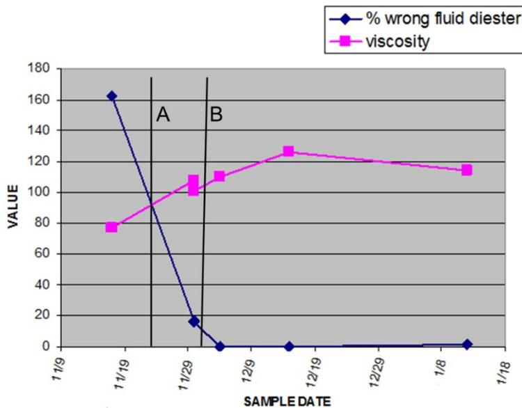
Fig. 5. Measures of viscosity and wrong fluid in a diesel engine. At Point “A”, the engine was replaced based on PFA analysis. At that time, the system oil was replaced. At Point “B”, the engine oil was replaced a second time.
