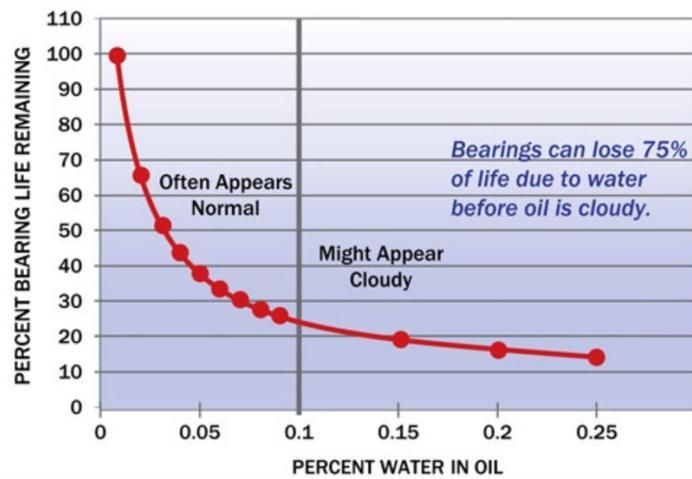
Fig. 4. Dependence of bearing life on concentration of water in lubricating oil as described in Ref 3. Reprinted with permission.
