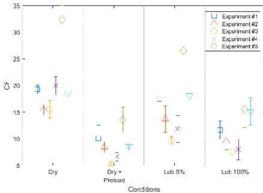
Figure 4: Crest Factor Performance Comparison for Experimental Conditions.
