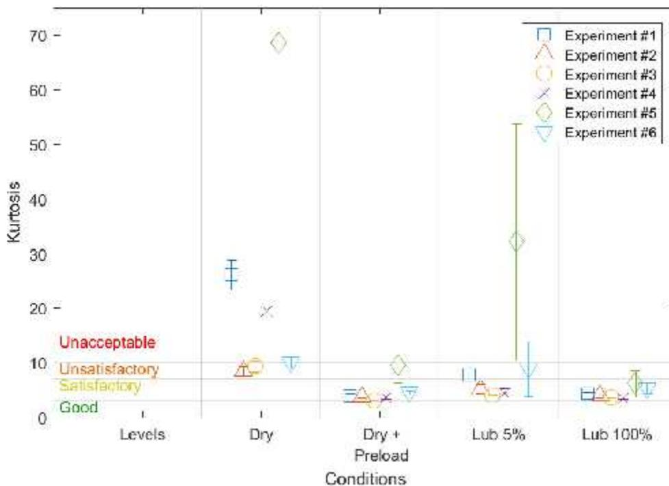
Figure 5: Kurtosis Performance Comparison for Experimental Conditions with Severity Levels.
