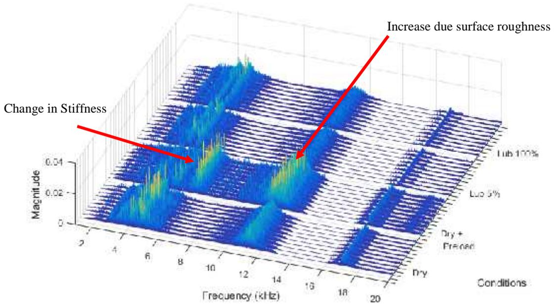
Figure 3: Cascade Comparison and Preload Effects on Experiment #2.
