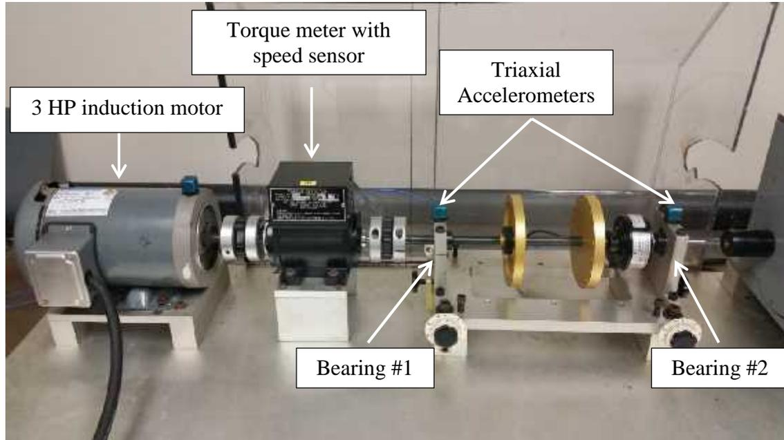
Figure 1: Test Bench Used for Experimentation.
