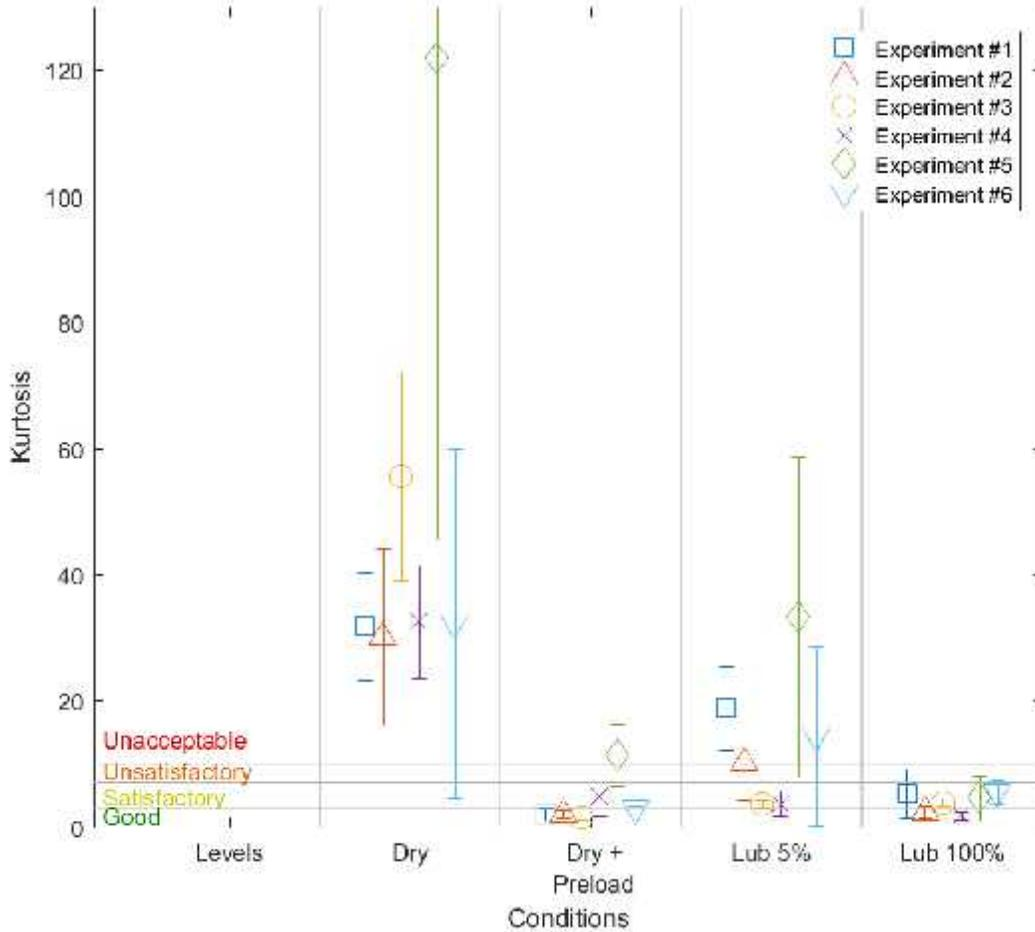
Figure 7: Kurtosis of Filtered Frequency Band Localized by Kurtogram.
