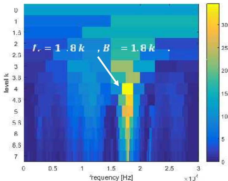
Figure 6: Fast Kurtogram for Experiment #1 on Dry Conditions.
