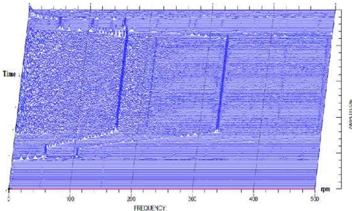
**Fig 3 – Low frequency Sub-synchronous vibration**
