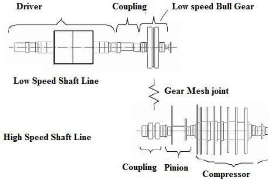
**Fig -1 - Torsional Model of a turbo compressor train**
