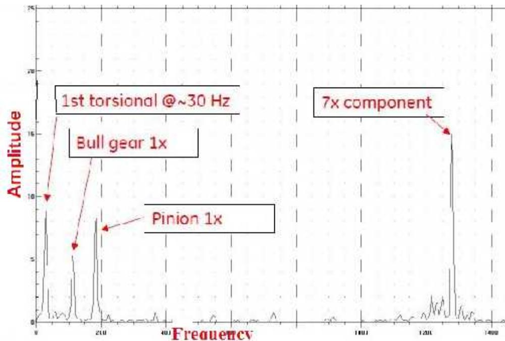
**Fig 5 – Pinion super- synchronous vibration**
