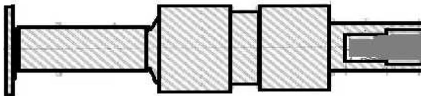
**Fig10- Tuning of pinion by removing mass ( temporary plug inserted)**
