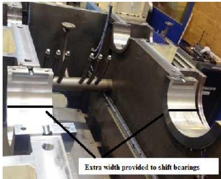
**Fig 8 - Gear Box bearing housing**
