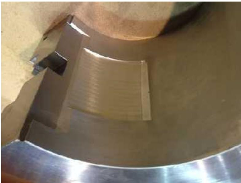
**Fig 4 - Relief created in pad to avoid sub synchronous vibration**
