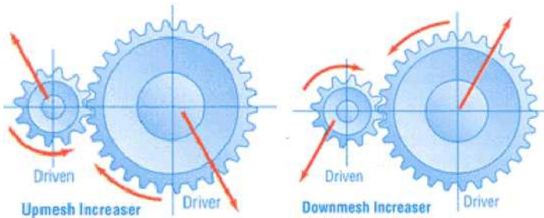
**Fig 2 Gear mesh force vectors**
