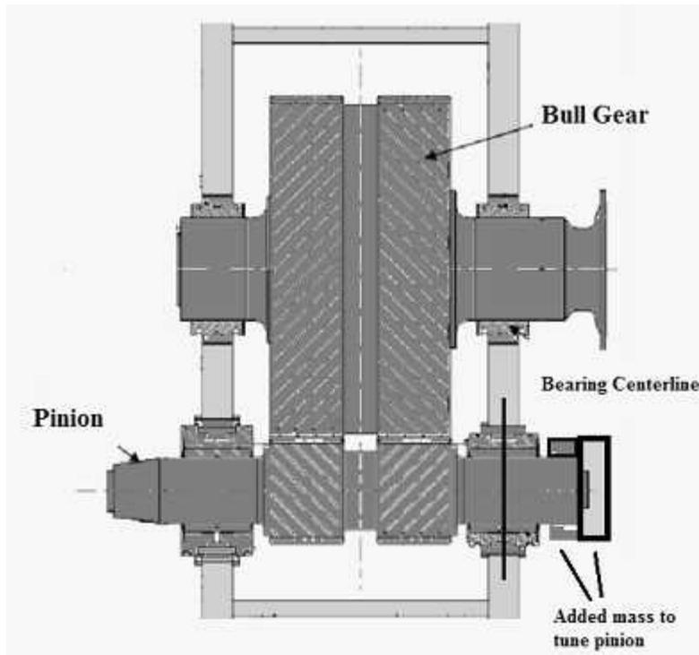
**Fig -9 - Tuning of pinion by adding mass**
