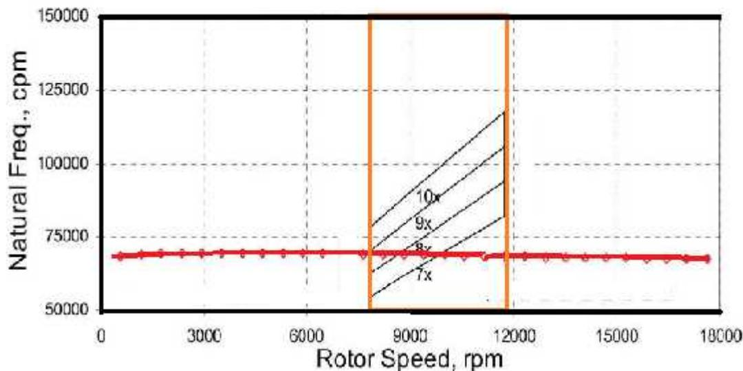
**Fig 7 - Identification of corresponding harmonics and 4th lateral frequency**
