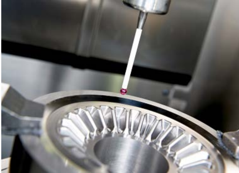
Fig 4 - Typical Coordinate measurement machine
