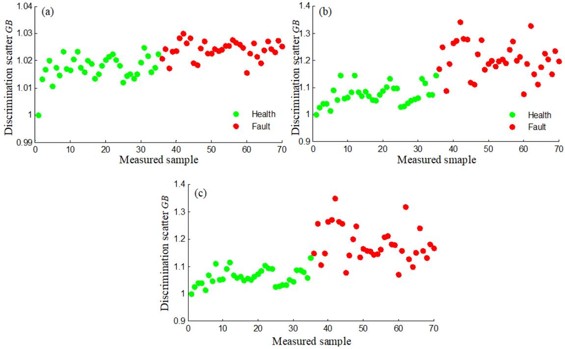
Figure 5. The health distribution of the measured Data A based on the proposed  $HI_{GM}$  with different kernel operation: (a)  $GB$ -Binet-Cauchy kernel, (b)  $GP$ -projection kernel and (c)  $GC$ -correction pseudo kernel.
