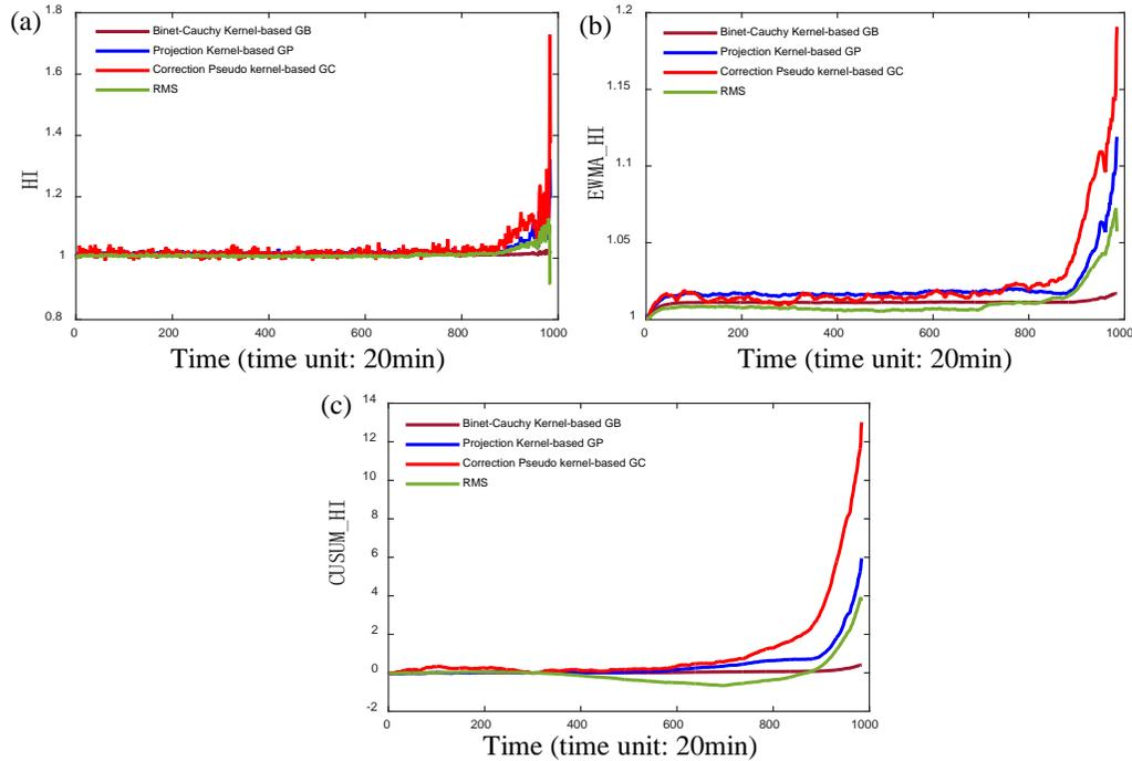
Figure 10. The PDA results for the full cycle life of the tested bearing 4#: (a) the raw HI, (b) the EWMA-based  $HI_w$  and (c) the CUSUM-based  $HI_c$  (the brown, blue, red and green lines represent different HIs, GB, GP, GC, and RMS, respectively).
