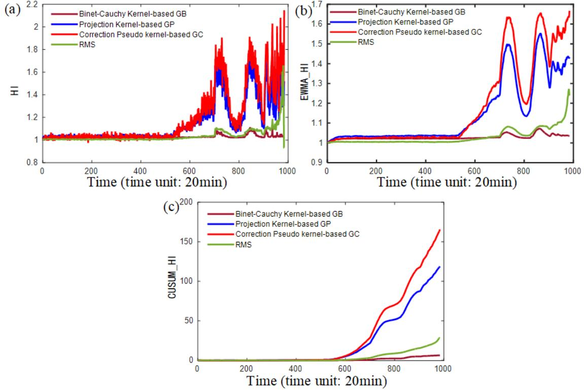
Figure 9. The PDA results for the full cycle life of the tested bearing 2#: (a) the raw HI, (b) the EWMA-based  $HI_w$  and (c) the CUSUM-based  $HI_c$  (the brown, blue, red and green lines represent different His, GB, GP, GC and RMS, respectively).
