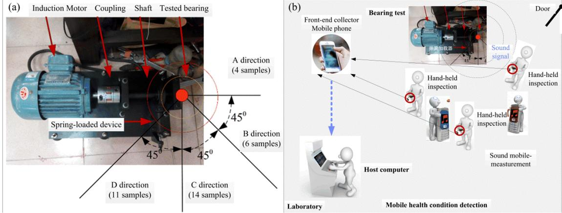
Figure 3. Experimental setup and mobile measurement for acoustic signal acquisition of ball bearing with outer-race defect: (a) bearing test, and (b) sound mobile-measurement.
