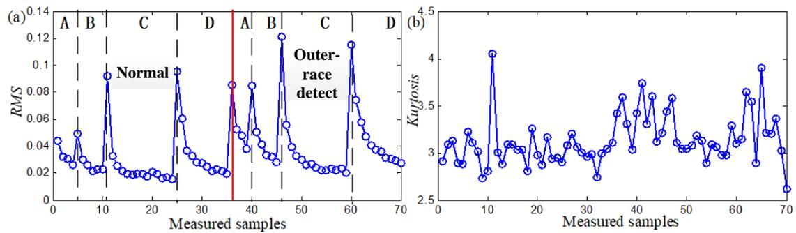
Figure 4. The health distribution of the measured Data A based on different HIs for Data A: (a) RMS and (b) Kurtosis.
