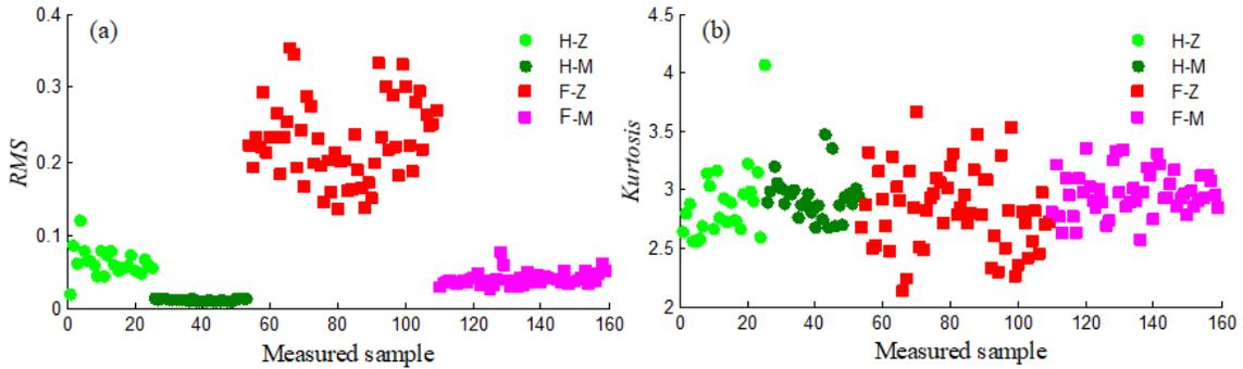
Figure 6. The health distribution of the measured Data B based on different HIs: (a) RMS and (b) Kurtosis.
