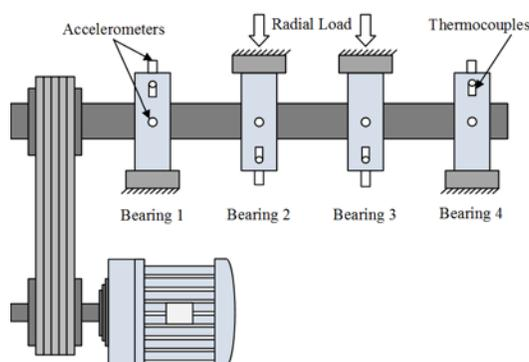
Figure 8. Bearing test rig
