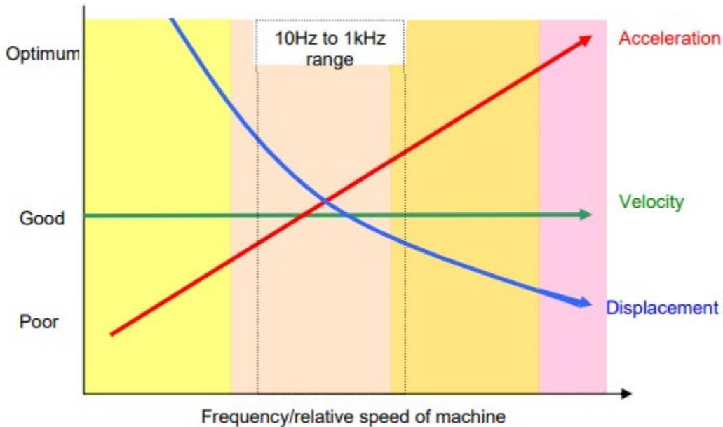
**Fig 5 – Range of various measurement accuracy of vibration and trade-off**
