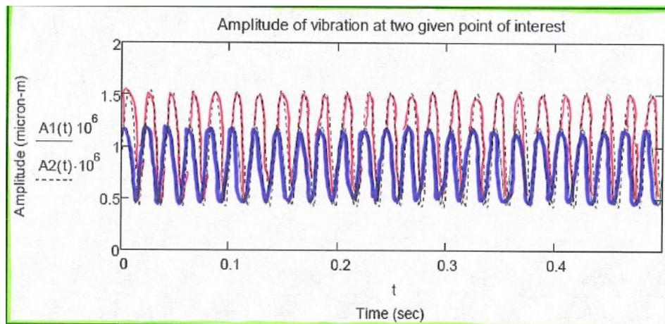
**Fig 8 Foundation analysis Output file for actual amplitude**
