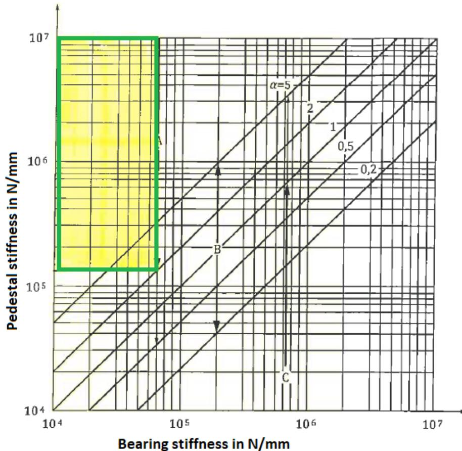
**Fig 10 -Zone of measuring relative shaft vibration based on stiffness ratio**
