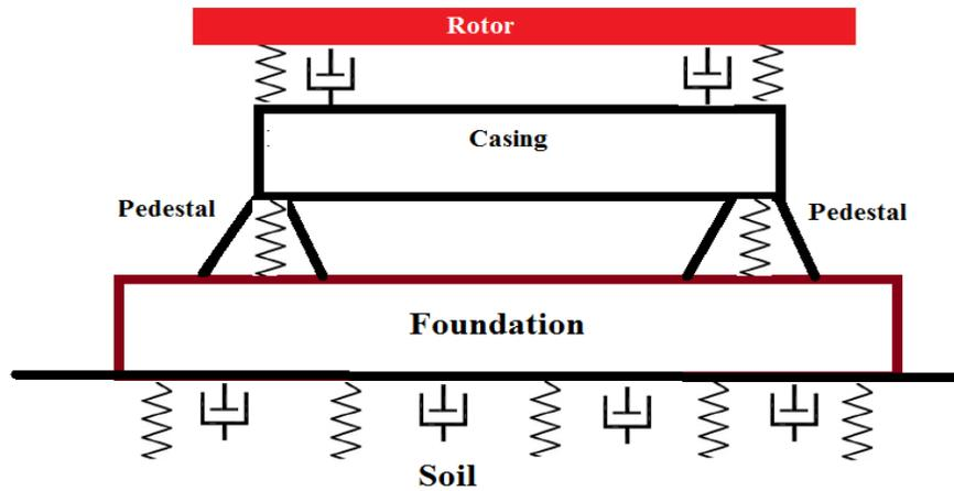
**Fig 6 -Transmission of vibration to foundation -rotor with hydrodynamic bearings**
