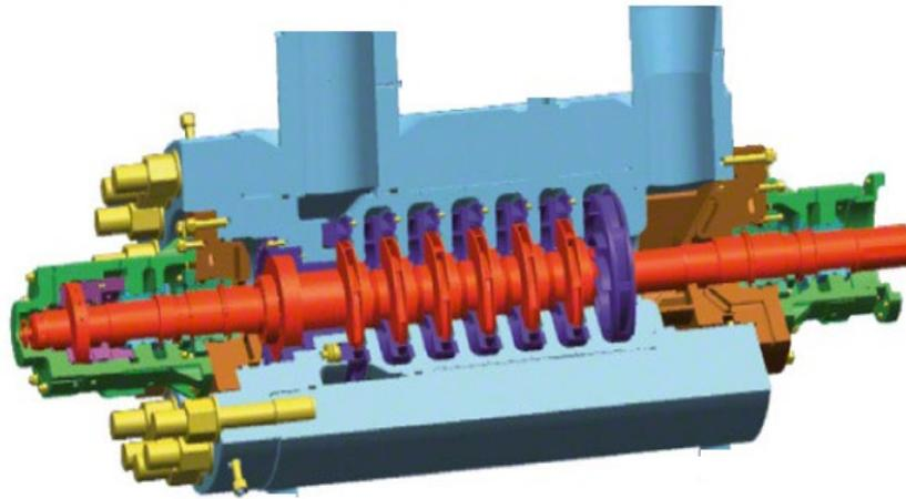
**Fig 9 - High speed turbo-machine Rotor (red) with highly stiff casing (in blue)**
