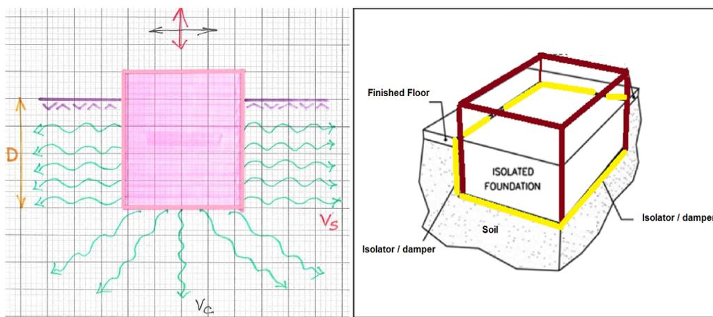
**Fig 3 -Shear & compression waves and dampening devices (shown in yellow)**
