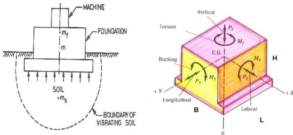
**Fig 1 Block type Foundation layout and rigid body modes**
